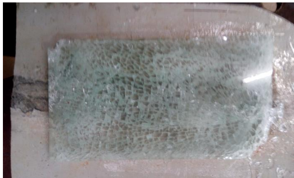
Tested Specimen after compression test
